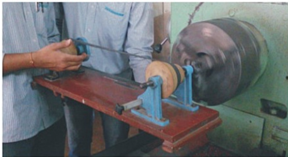
Working model of CVT
